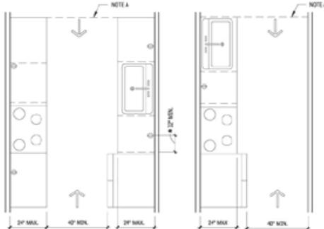
NOTE A: END WALL ONLY PERMITTED IN ICC/ANSI A117.1 (TYPE A AND TYPE B UNITS), AND FMBC UNITS IF WIDTH IS LESS THAN 60 IN (67 IN IN ICC/ANSI A117.1-2018).
